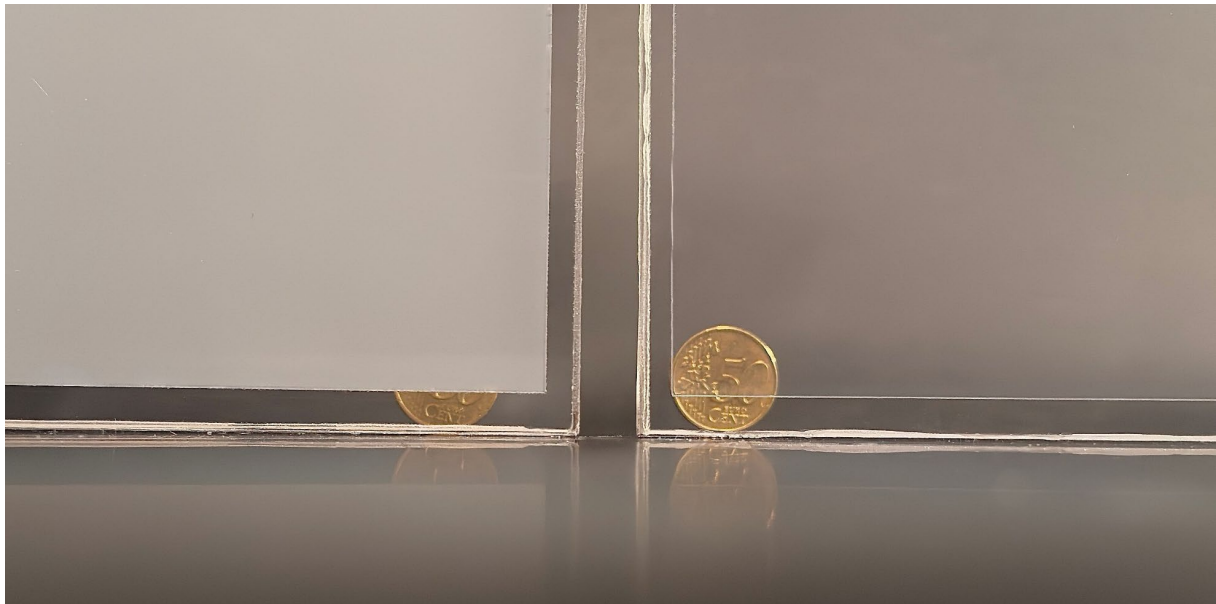
Fig. 5: Smart thin glass-polycarbonate composite panel in the opaque state (left) and transparent state (right).
