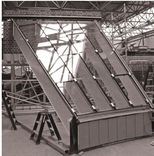
Figure 11: Full scale test assembly glass roof Victoria & Albert Museum.
