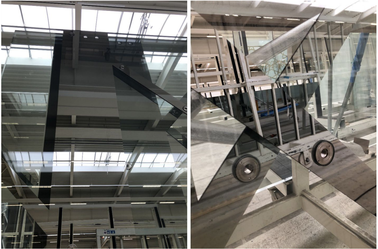
Fig. 26: Fabrication of the vertical glass with the Ipachrome coating, © sedak.
