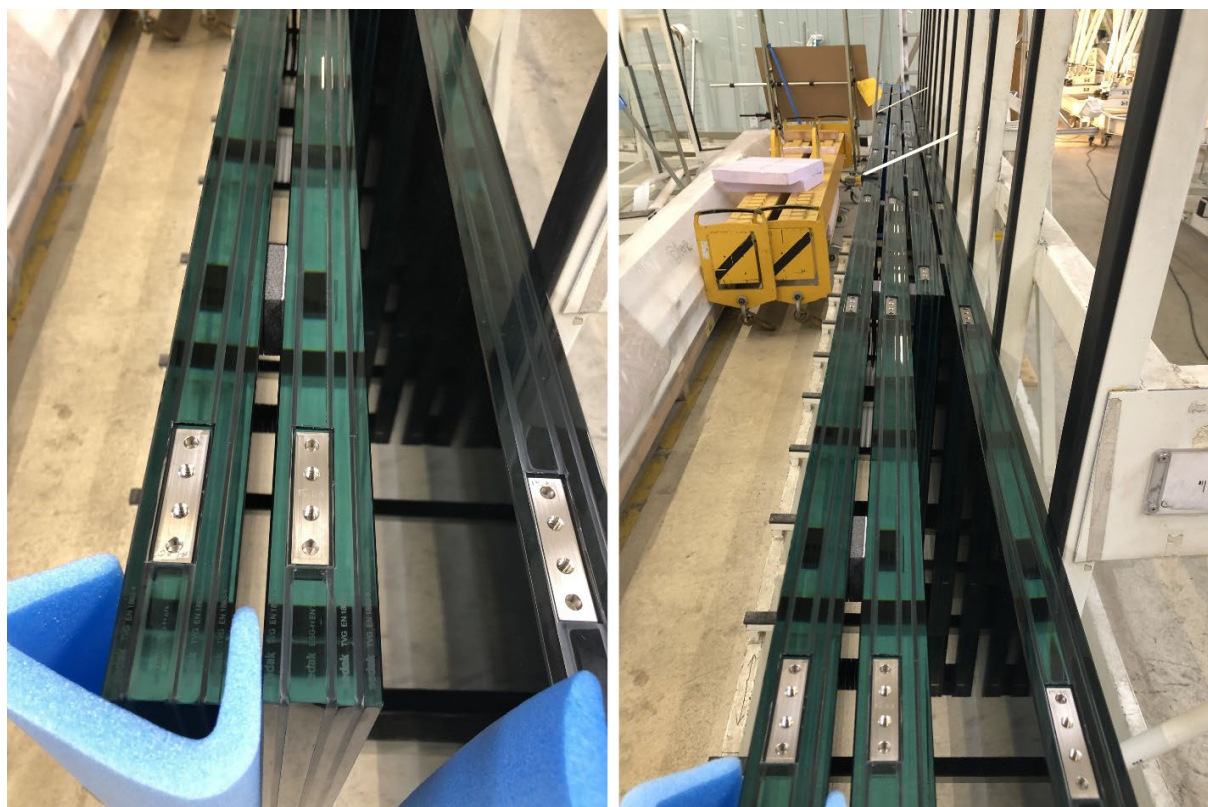
Fig. 25: Fabrication of the diagonal glass with the titanium inserts, © sedak.
