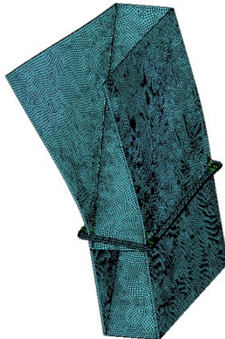
Fig. 14: Typical deflected shape under wind load (magnified x100), © Werner Sobek.
