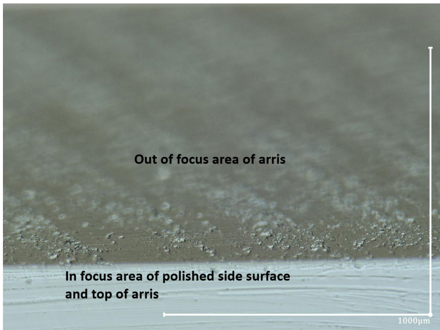
Fig. 3: Photo of edge of arris, magnification 200X, transmitted lighting.
