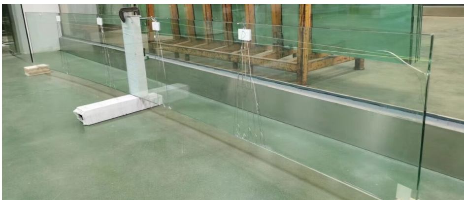
Fig. 14: Fracture pattern – Specimen set VT(8)
