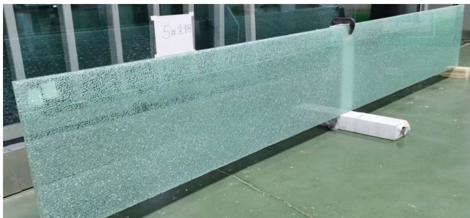
Fig. 16: Fracture pattern – fully toughened glass.
