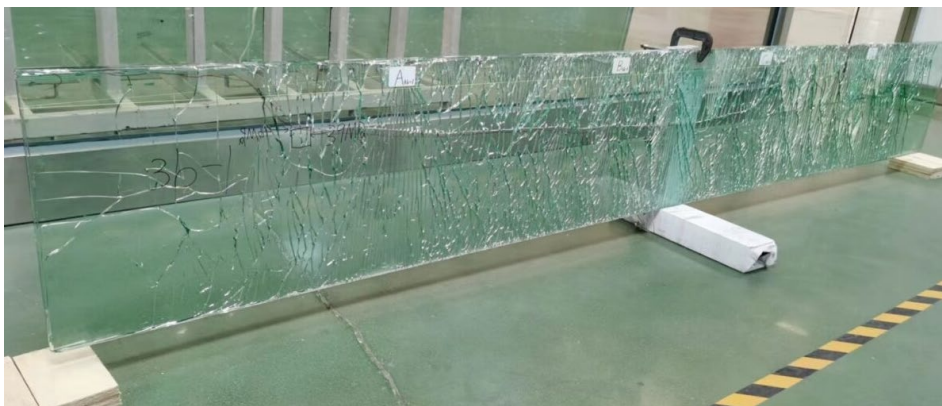
Fig. 13: Fracture pattern – Specimen set VT(12)
