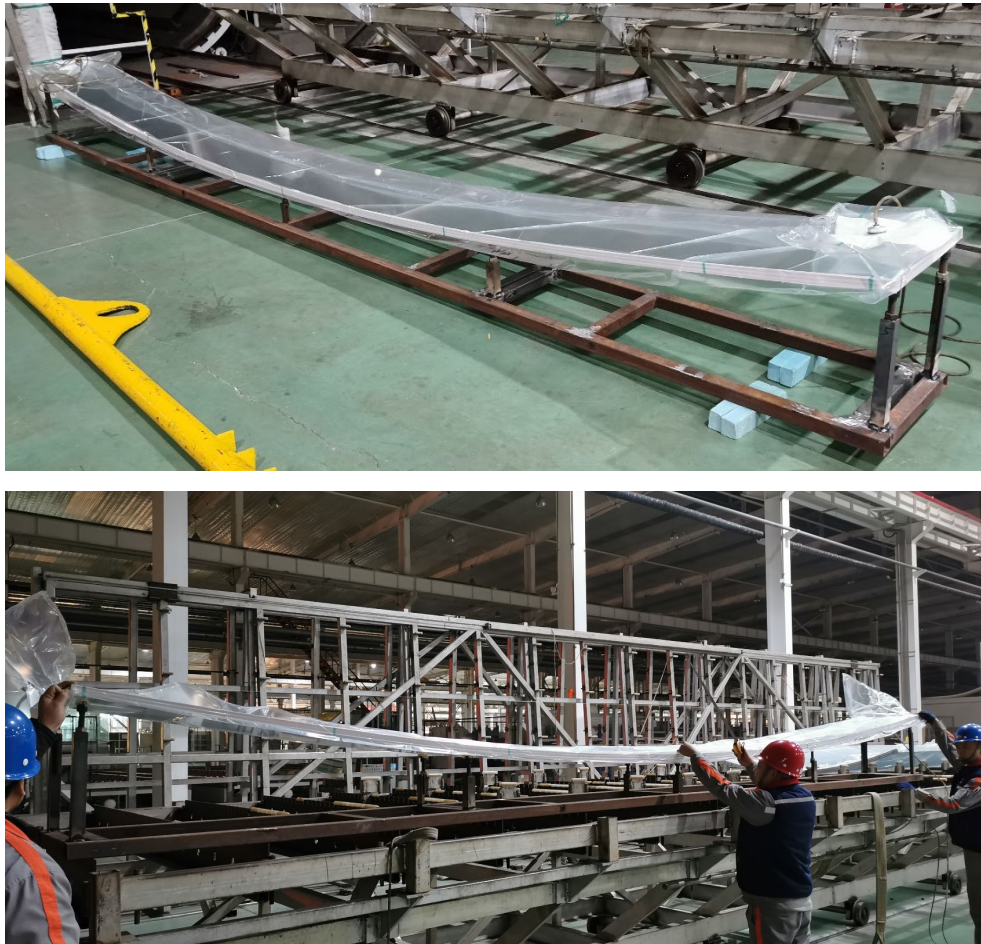
Fig. 3: Warm bent process of glass.
