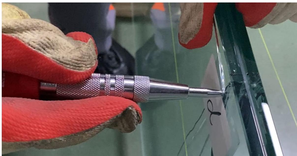
Fig. 6: Glass breaking by a centre punch.
