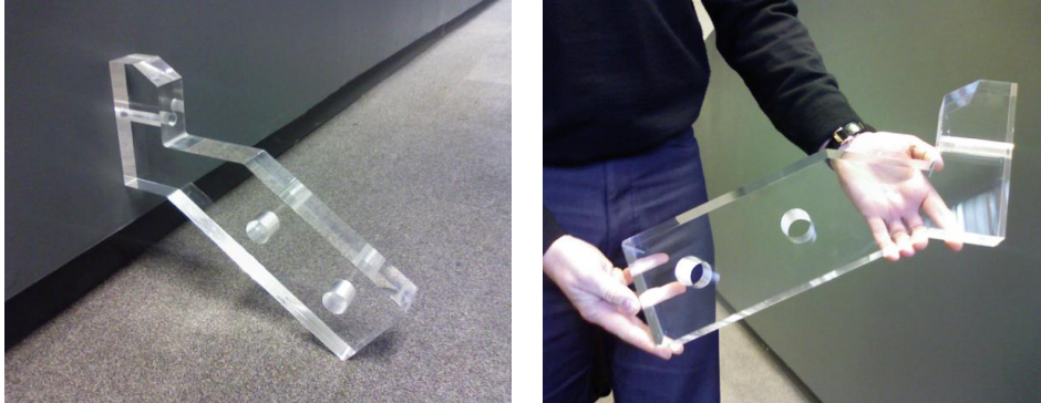
Figure 5: Prototype Acrylic Connection Joint between Rafter and Rafter Plate.
