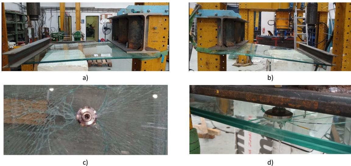
Fig. 6: a) The fractured specimen; b) The specimen after 48 hours; c) A detail of the fracture around the connection; d) The spider-shaped fracture.
