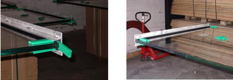
Figure 7: Adhering aluminum profile to glass panes.
