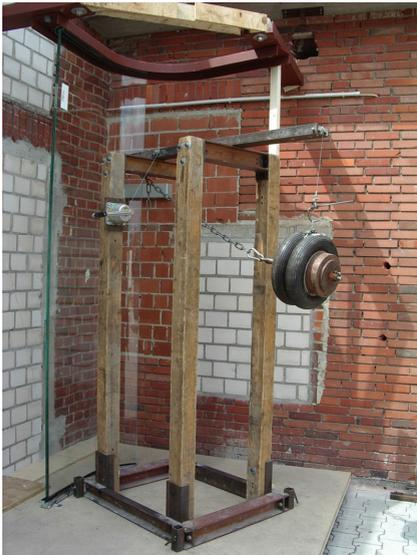
Figure 6a: Construction of pendulum impact test.
