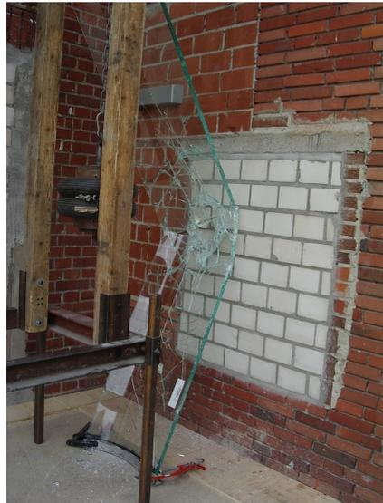
Figure 6b: Collapsed glass unit.
