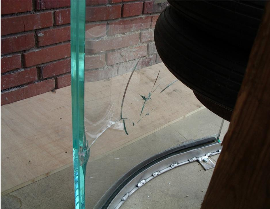
Figure 5: Hitting the inner pane at the edge before impact test and breakage effected by impact.
