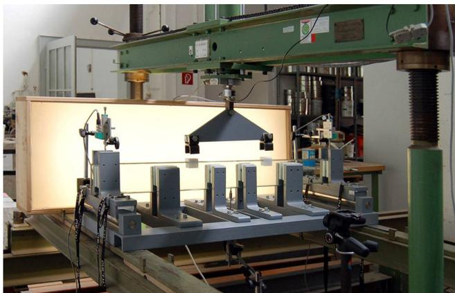
Figure 1: Experimental setup of four-point bending test.
