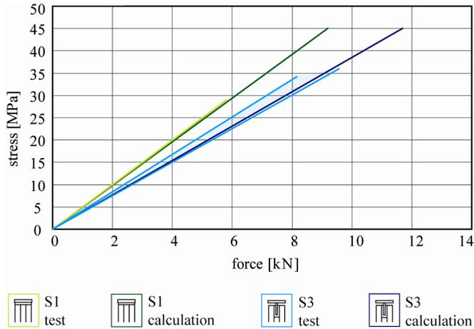
Figure 7. Comparison of the experimental force-stress diagram with the results of the numerical simulation.
