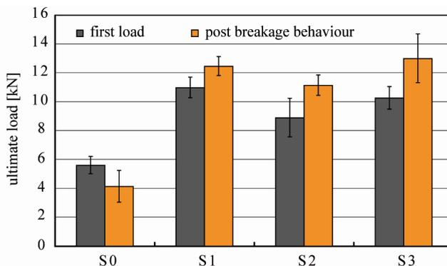
Figure 5: Ultimate load of the hybrid beams.
