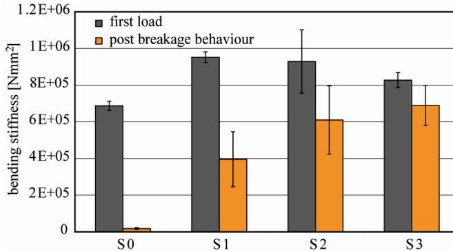
Figure 6: Bending stiffness of the tested beams.
