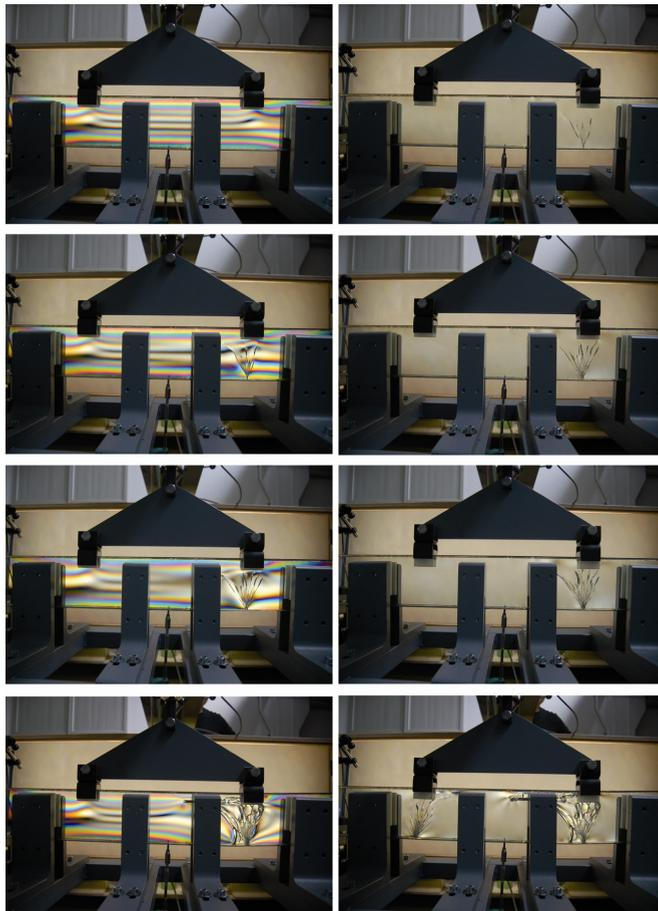
Figure 3: Changes of stress during loading.
