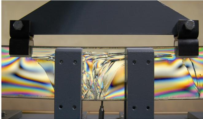
Figure 4: Crack pattern of a hybrid beam after breakage of all panes.
