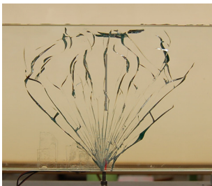
Figure 6: Typical glass fracture pattern in a composite beam.
