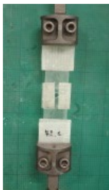
Fig. 6: GFRP reinforced open hole test specimen (note: GFRP strips were also used to reinforce the ends of test specimen as means of eliminating possible failure at the ends of the test specimen)
