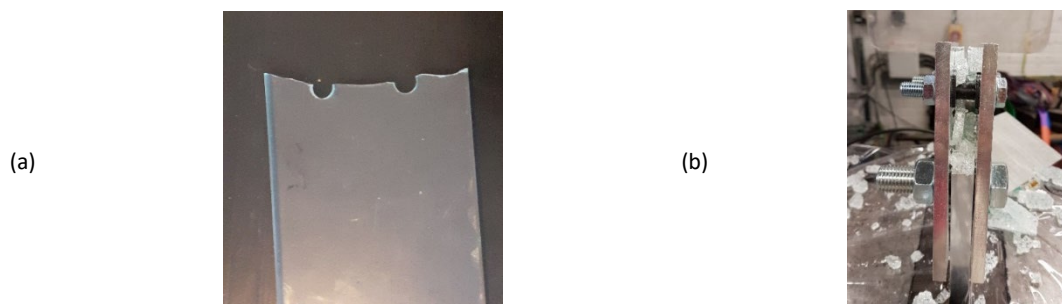
Fig. 2: Typical failure modes of: (a) annealed glass and (b) tempered glass-bolted joints
