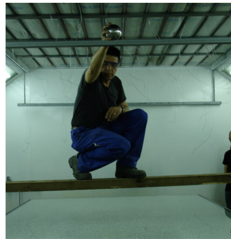
Figure 9: Hard-body impact test included in the CWCT-42 test sequence.
