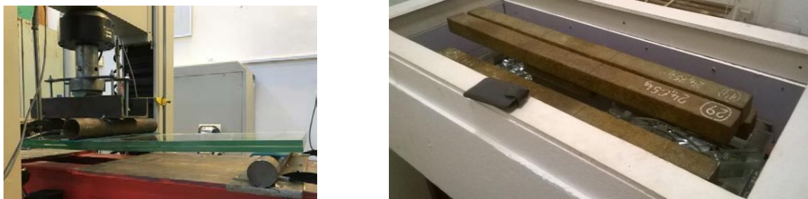
Fig. 8a) Panel loaded in displacement controlled bending test, b) Panel loaded in bending creep test – opened chamber right after loading
