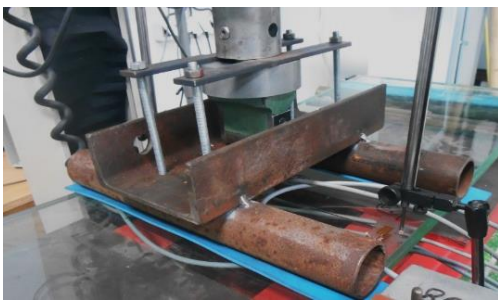
Fig. 6a) Loading apparatus in displacement-controlled test, b) Loading apparatus in creep tests.
