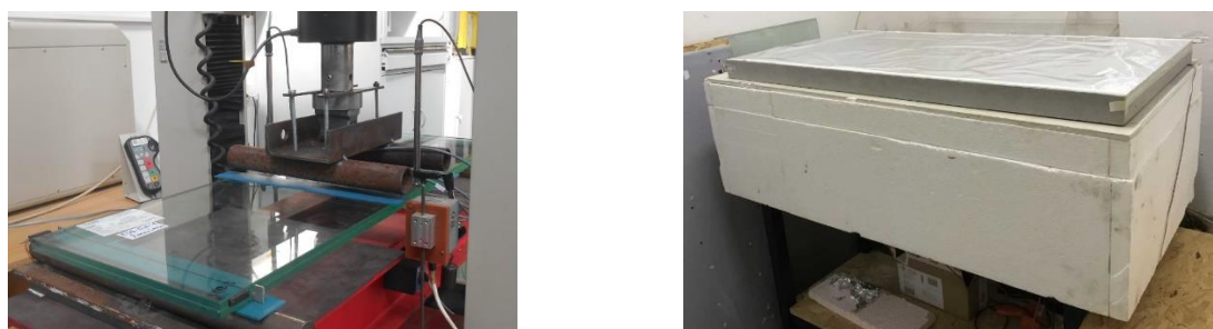
Fig. 1a) MTS loading device for displacement-controlled tests, b) Closed climatic chamber for creep tests ensures climatic conditions.
