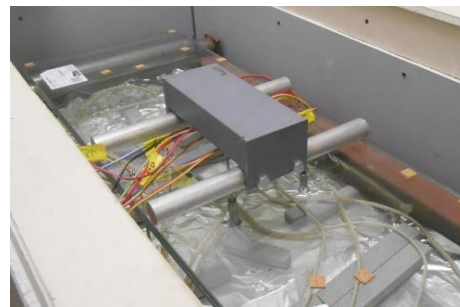
Fig. 6a) Loading apparatus in displacement-controlled test, b) Loading apparatus in creep tests.
