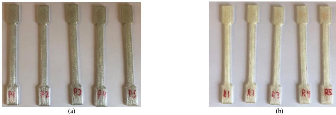
Fig. 4a) UV ageing of 3D printed PET specimens after two weeks, b) UV ageing of 3D printed recycled PET specimens after two weeks
