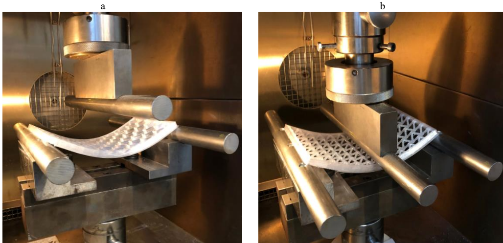
Fig. 12a) Recycled PET core with honeycomb pattern deflection without a force at 80 °C, b) Recycled PET core with truss pattern deflection at 80 °C.
