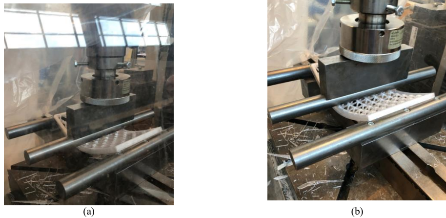
Fig. 10a) Honeycomb recycled PET core at a deflection of 50 mm, b) Truss recycled PET core at a deflection of 50 mm.
