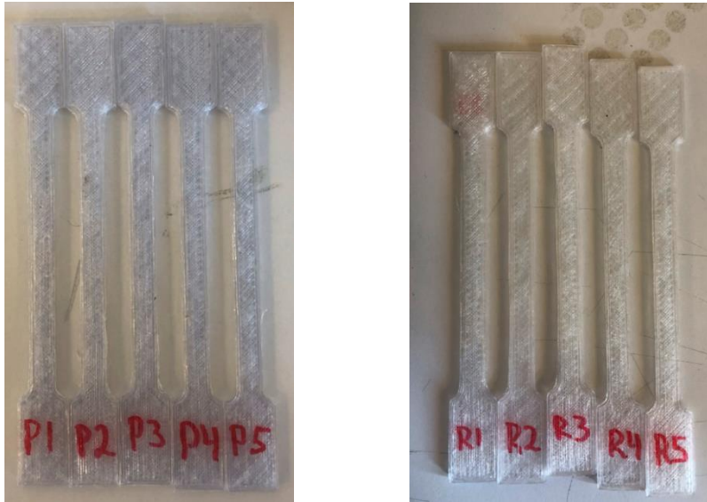
Fig. 2a) dimensions dumbbell specimens based on NEN-ISO 527-1 Standard, b) 3D printed PET specimens, c) 3D printed Recycled PET specimens.
