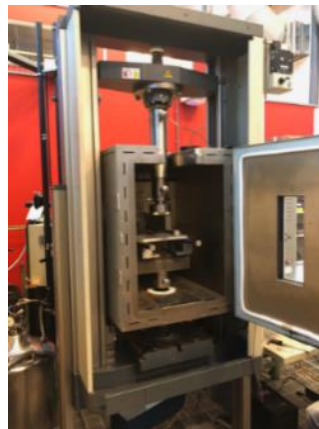
Fig. 11 3-Point bending test setup for elevated temperatures.
