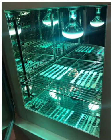
Fig. 3 Accelerated UV source with 3D printed specimens.
