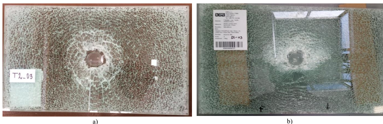
Fig. 13 a) Fractured tensile tests sample, b) fractured eccentric shear force tests sample.
