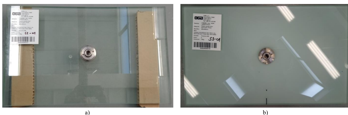
a) b) Fig. 2 a) Sample with a clear EVA foil, b) sample with an opaque EVA foil.
