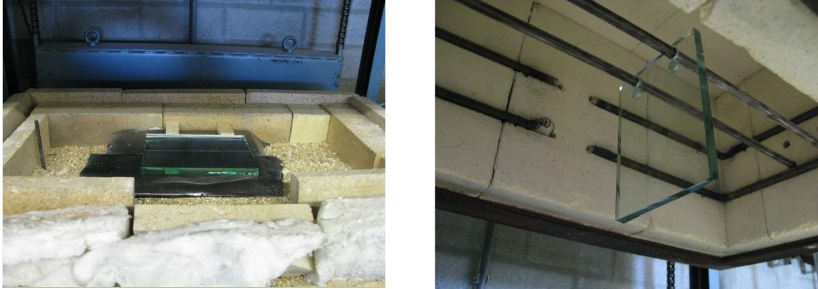
Fig. 4 Welding experiment, the position of the flange (left) and the web suspended in the box oven (right) prior to preheating.
