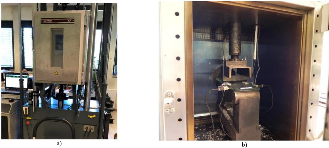
Fig. 5 Environmental chamber a) and three-point bending test setup prepared in the environmental chamber b) to ensure elevated temperature during the test.
