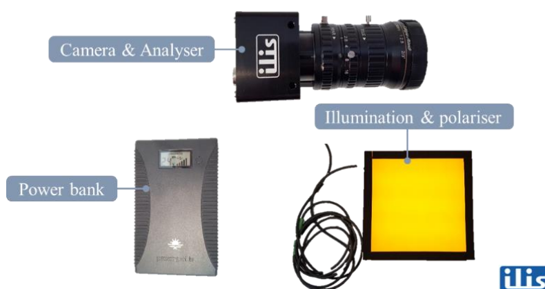
Fig. 6 Components of the mobile measuring device.
