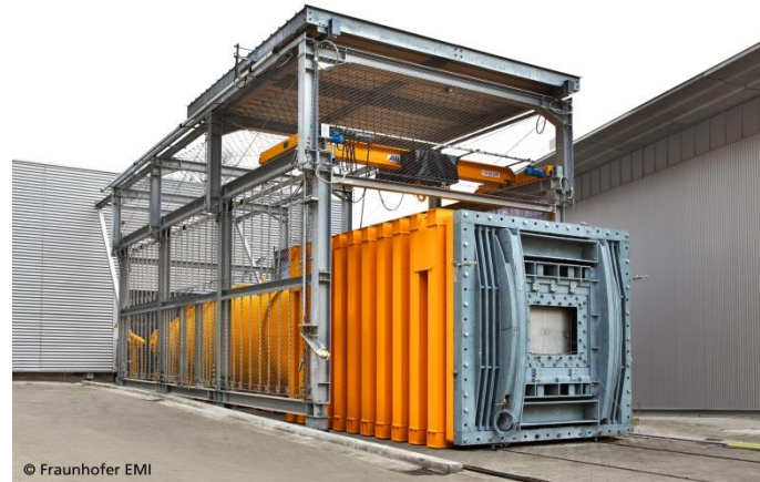
Fig. 1 Blast-star shock tube at the Fraunhofer EMI site in Efringen-Kirchen.
