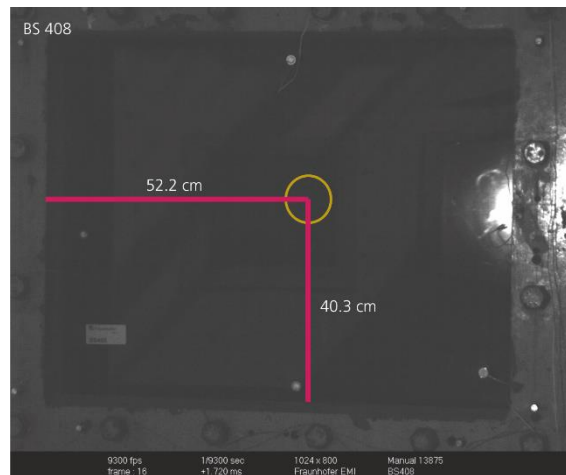
Fig. 6 Visually determined location of initial crack formation using high-speed video recordings (BS 408).
