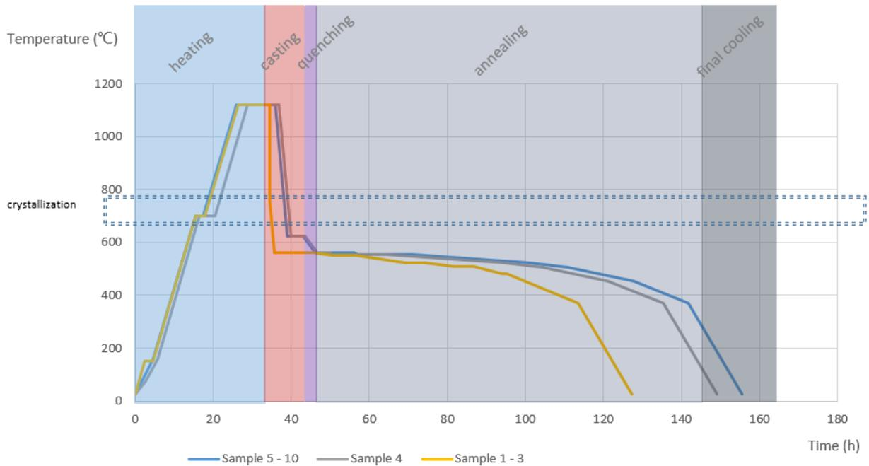
Fig. 3 The firing schedule for three kiln casting.
