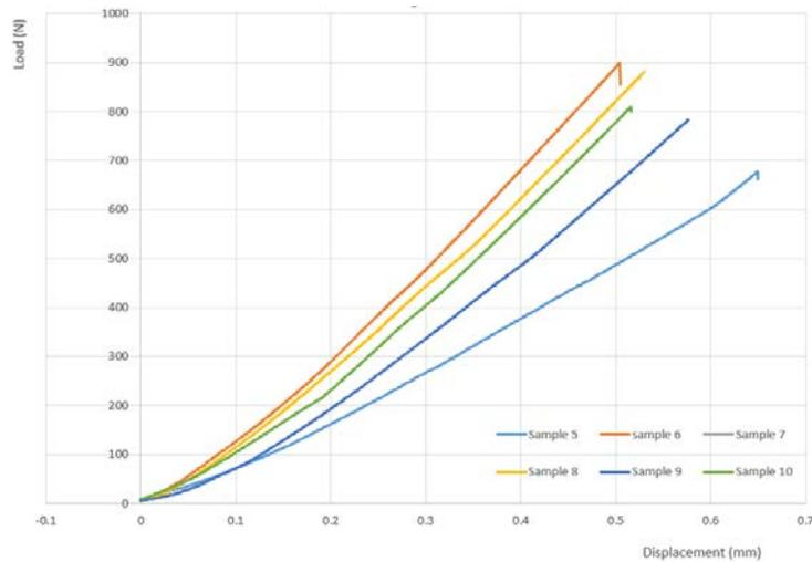
Fig. 16 The load-displacement curve for sample 5 to 10.
