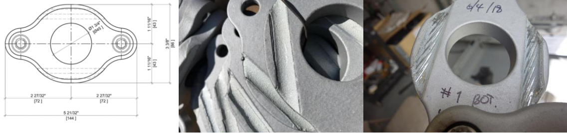
Figs. 25, 26, 27 Drawing of a cable clamp (left), fabricated pieces with special zinc coating in the notched steel (center), and tested clamp assembly with visible traces of the cable wires (right). All images: Knippers Helbig.
