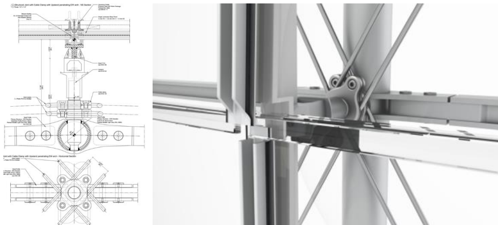
Figs. 14, 15 Typical Glazing detail 2D and 3D (Images: Knippers Helbig).
