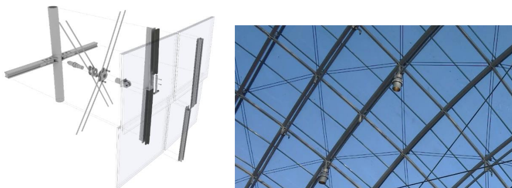
Figs. 4, 5 Explosion diagram study of the structural + glazing build up (left) and the installed detail on site (right). Graphic and Image: Knippers Helbig.
