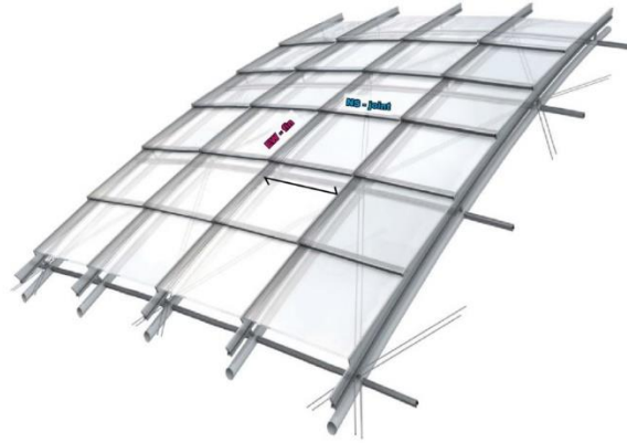
Fig. 13 3D diagram of the shingled glazing system. Image: Knippers Helbig.
