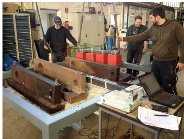
Fig. 4 Test panel under load.
