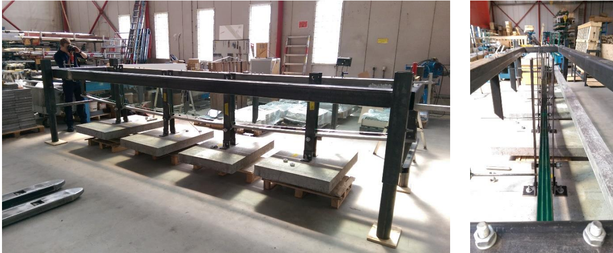
Fig. 9 Right, Sample 2 – 2.5xULS302. Left, lateral deflection under the loads is monitored via a displacement gauge [Octatube].
