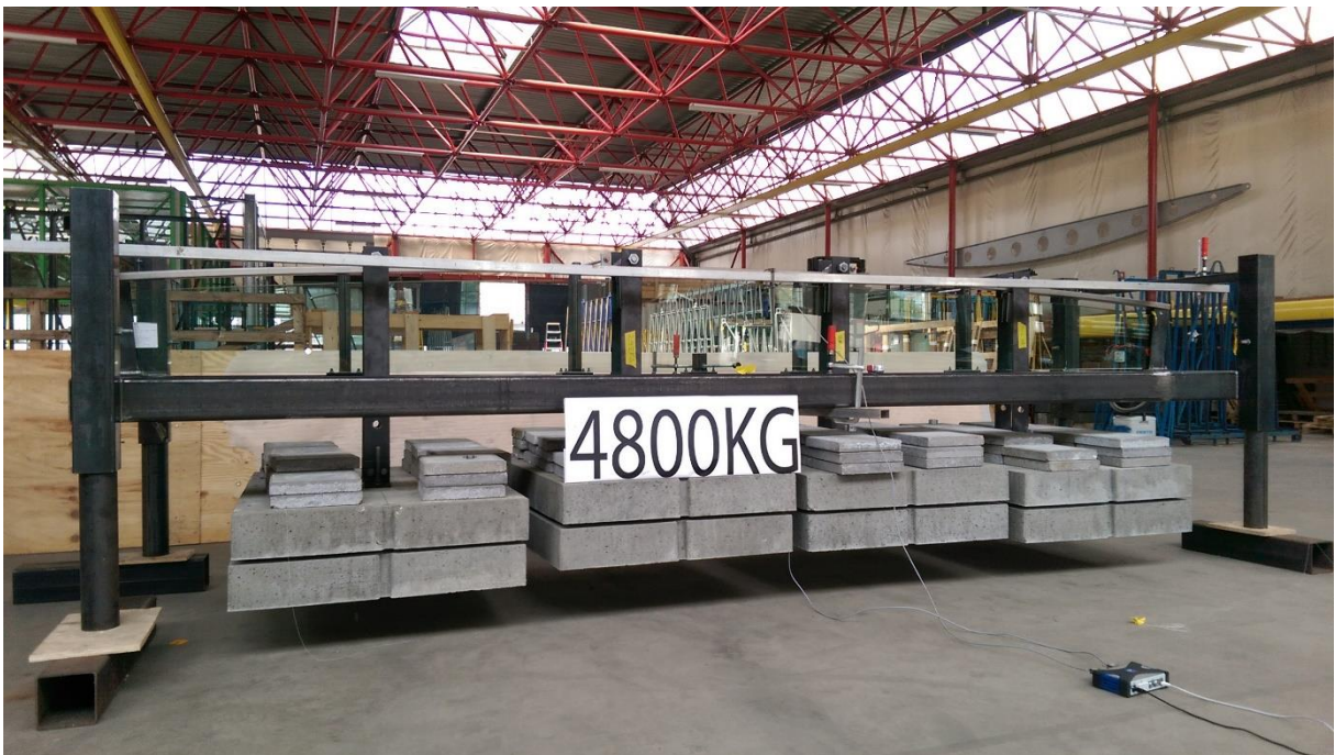
Fig. 8 Sample 1 – 2.5x ULS301= 4800 kg [Octatube].
