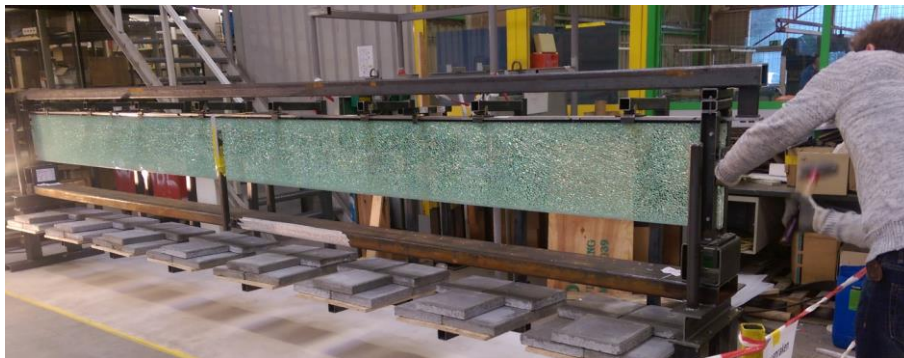
Fig. 17 Fin with two broken glass sheets, post failure behavior.
