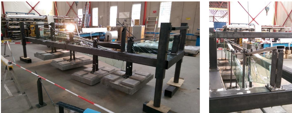
Fig. 12 Sample 1 – Post breakage failure [Octatube].
