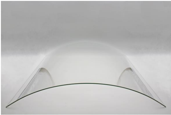
Fig. 1 Cold-bent thin glass during lamination process (Kloker 2012, © seele).
