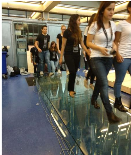
Fig. 13 Non-destructive test of large prototype panel using dynamic load.
