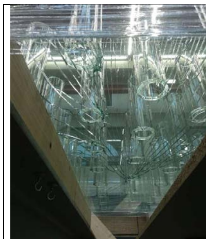
Fig. 19 cracks in bottom plate originating from a spacer.
