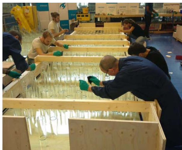
Fig. 11 applying adhesive to top of cylinder before placing top panel.
