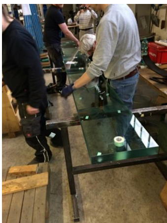
Fig. 8 Glass fin splice testing.
