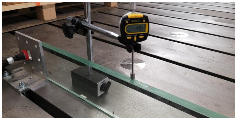
Fig. 5 Measuring the offset with a dial gauge.
