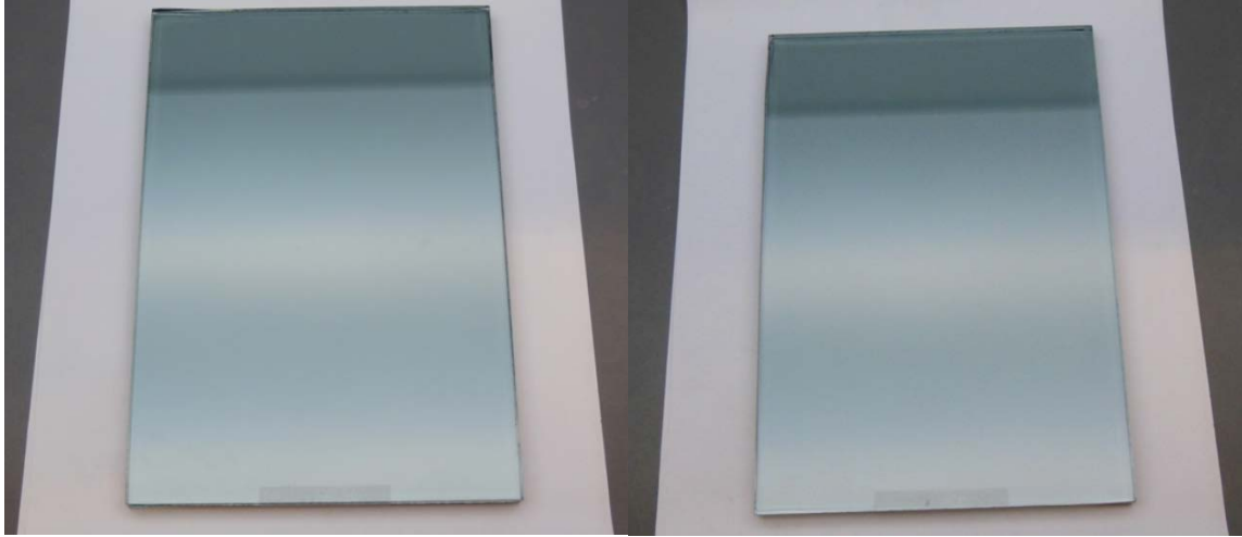
Fig. 4. Photograph of coating E, in position #2 (left side) and position #4 (right side) (illuminant D65 on white paper)
