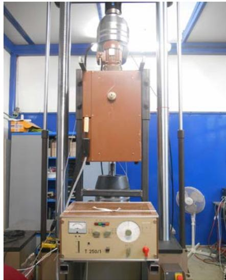
Fig. 4 MTS 500B with TiraTest 201 chamber for DMTA.
