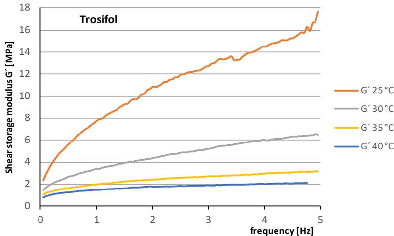
Fig. 10 Storage modulus-frequency curves of representative Trosifol interlayer obtained by DMTA.
