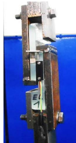
Fig. 2a) Specimen with potentiometric linear transducers, b) Specimen fixing in metal jaws (TIRA, MTS).
