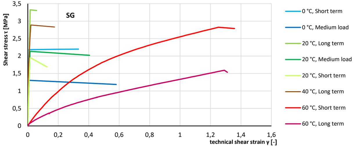
Fig. 9 Representative stress-strain curves for SG interlayer.
