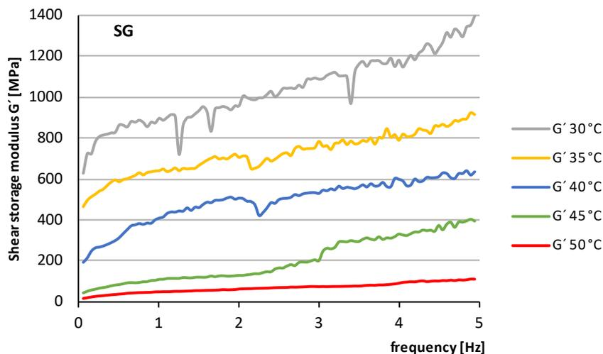
Fig. 11 Storage modulus-frequency curves of representative SG interlayer obtained by DMTA.
