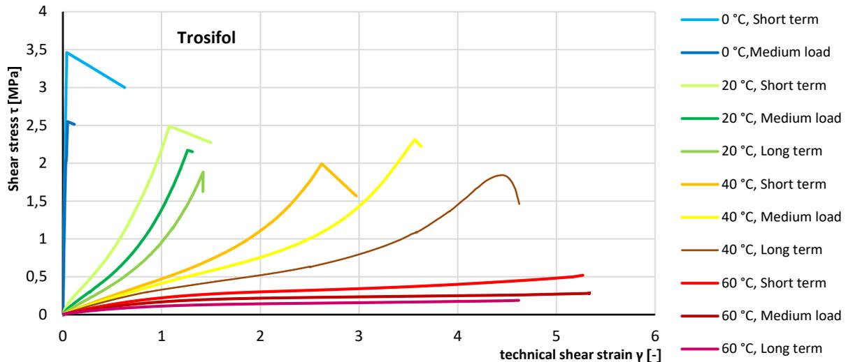
Fig. 8 Representative stress-strain curves for Trosifol interlayer.
