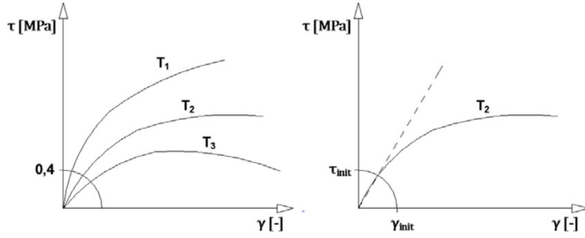
Fig. 6 Initial shear modulus evaluation where the temperatures  $T_1 > T_2 > T_3$ .
