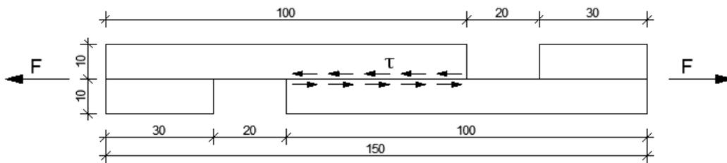
Fig. 1 Nominal dimensions of the testing specimen.
