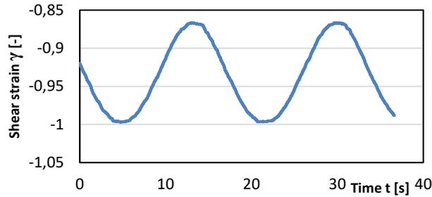
Fig. 3 Shear strain example of the interlayer during DMTA.
