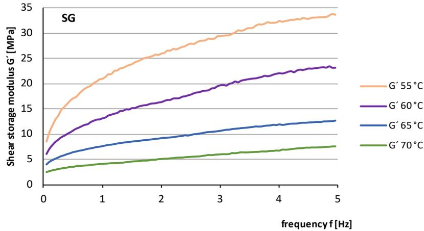
Fig. 12 Storage modulus-frequency curves of representative SG interlayer in high temperatures obtained by DMTA.
