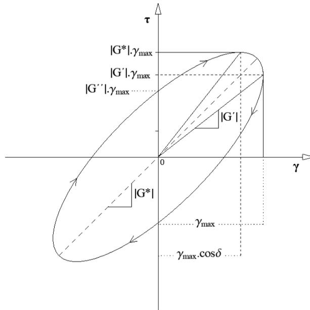
Fig. 7 Hysteresis loop showing stress-strain dependence in each loading cycle with its important points, (Lakes 2009).
