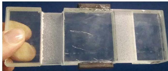
Fig. 14 Trosifol delamination, sample dynamically loaded at 40 °C.
