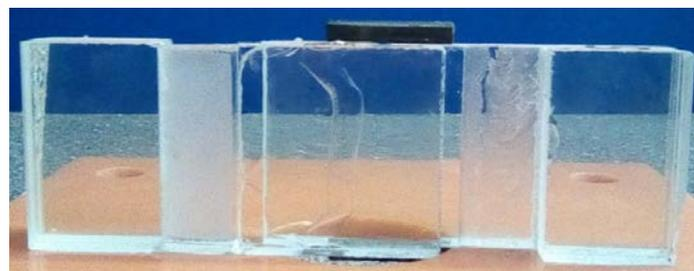
Fig. 15 SG delamination, sample dynamically loaded at 75 °C.
