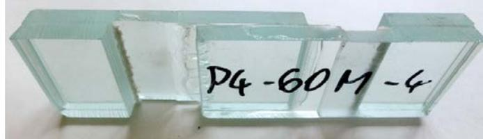
Fig. 13 Trosifol delamination, sample statically loaded at 60 °C.
