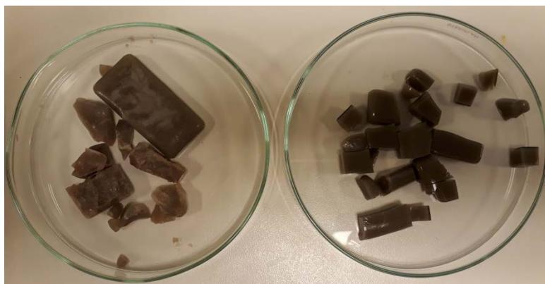
Fig. 3 Non-transparent samples containing 80KPO<sub>3</sub>-20Slag and 70KPO<sub>3</sub>-30Slag, respectively.
