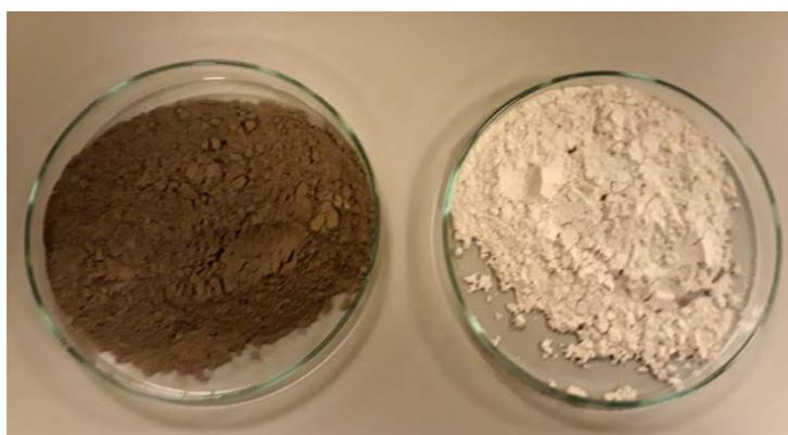
Fig. 2 The raw waste materials, fly ash and slag.
