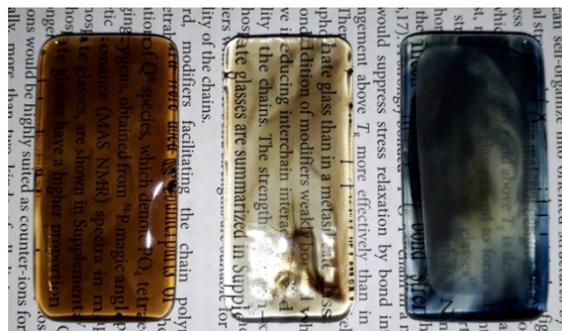
Fig. 6 Samples consisting of 15% slag, without the addition of B<sub>2</sub>O<sub>3</sub>, with the addition of 10% B<sub>2</sub>O<sub>3</sub> and 20% B<sub>2</sub>O<sub>3</sub>, respectively.
