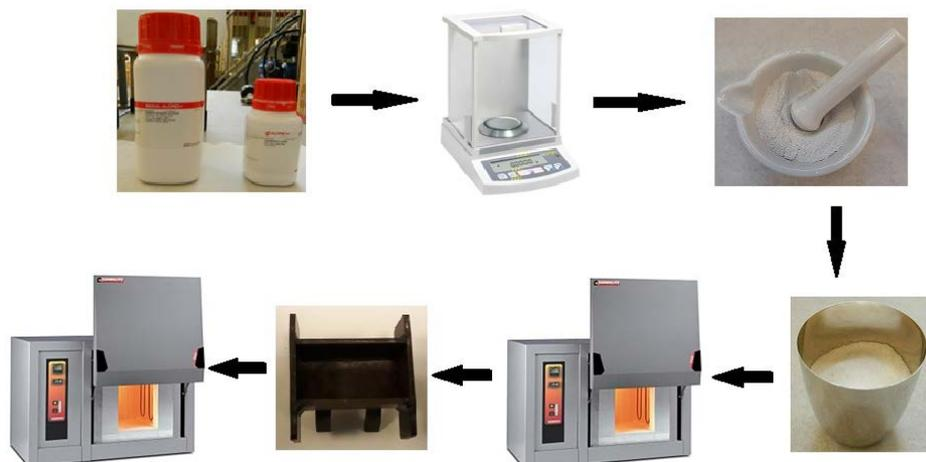
Fig. 1 Scheme of the glass samples production.
