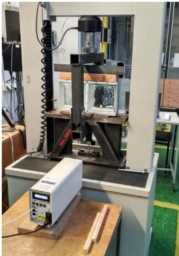
Fig. 17 The component "Anchoring of the reinforcement in tension" during the test.
