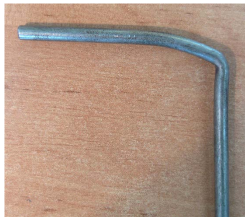
Fig. 18 Deformation and damage of the spacers and the reinforcement at anchoring (left), deformed reinforcing bar after the test (right).
