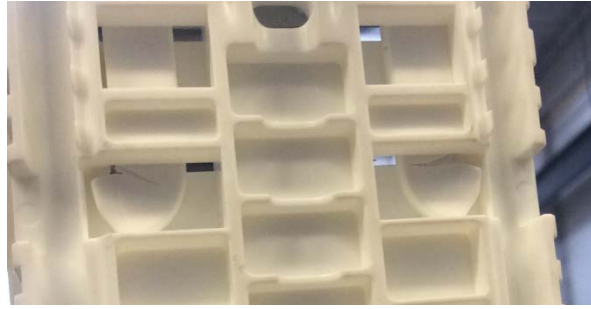
Fig. 12 The collapse mode of the component "Spacers and connector in tension".
