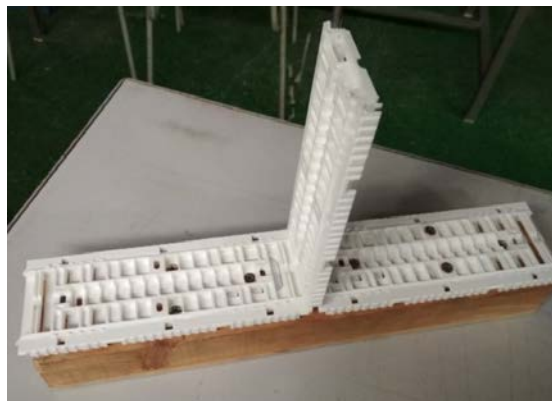
Fig. 16 The spacers are fixed to the timber frame.
