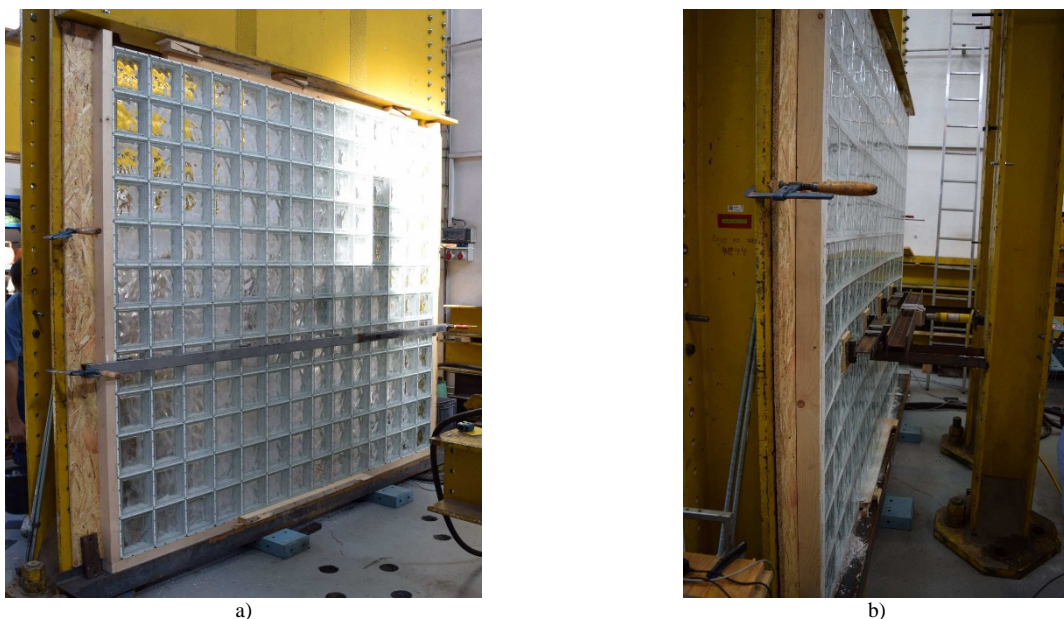
Fig. 5a) The completed wall prior to filling of the joints, b) deformed wall during the test.
