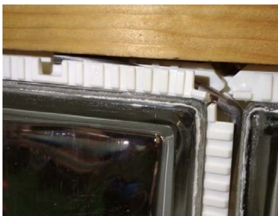
Fig. 18 Deformation and damage of the spacers and the reinforcement at anchoring (left), deformed reinforcing bar after the test (right).
