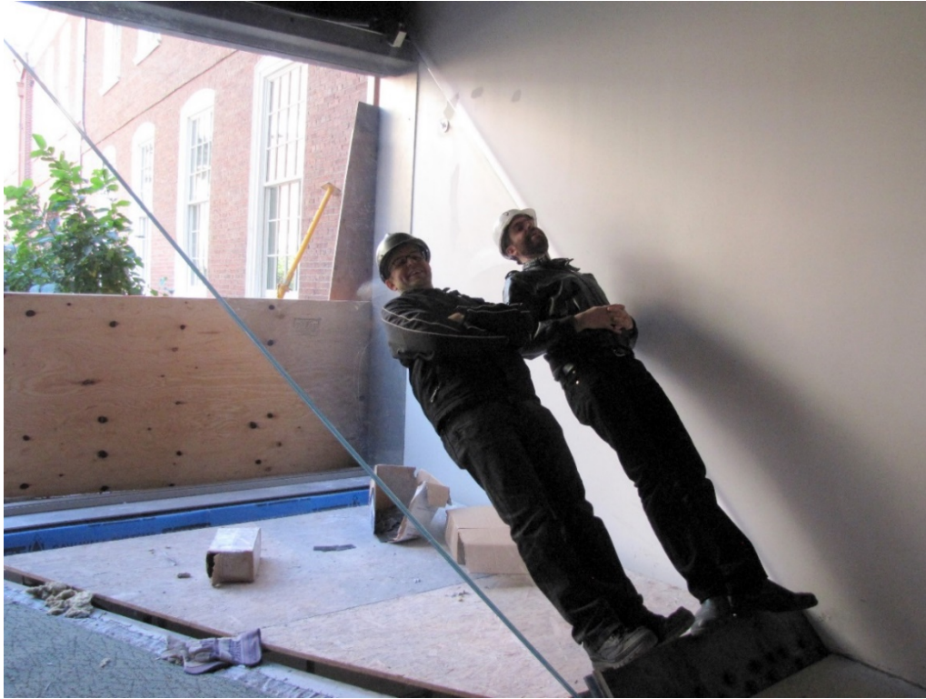
Fig. 10 P-131317, 2011 | Load testing of glass
