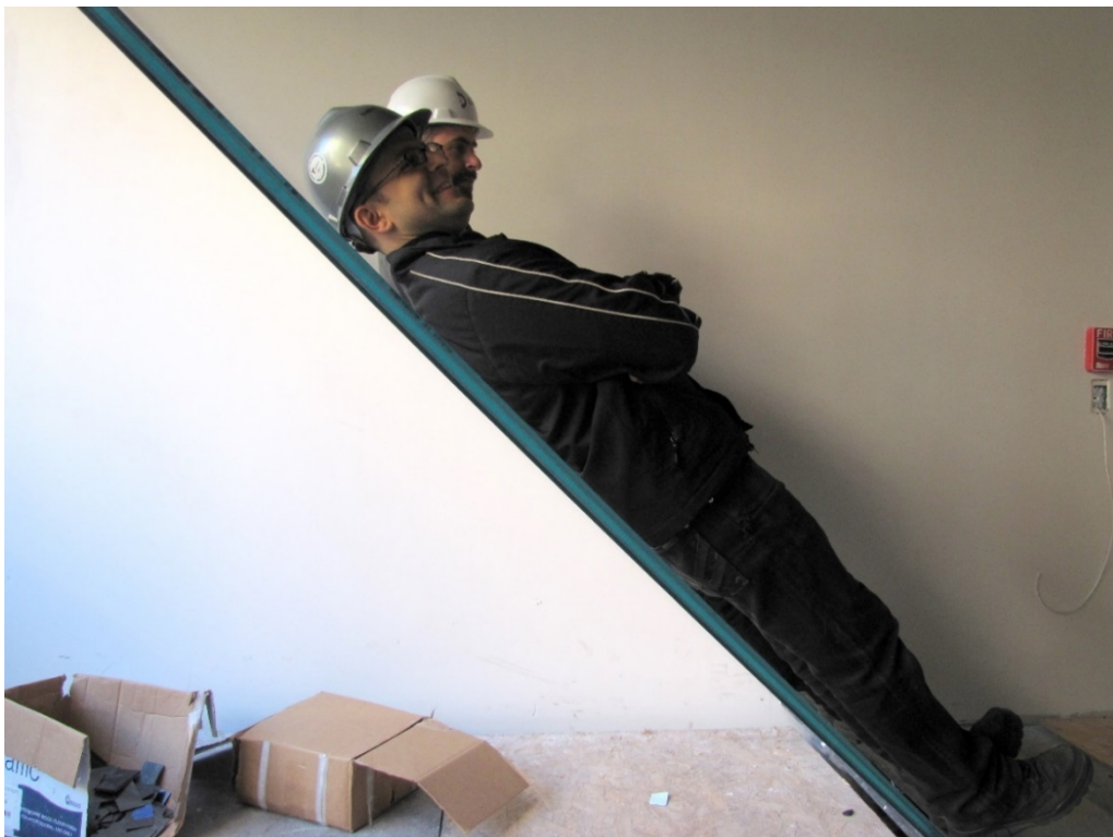
Fig. 11 P-131317, 2011 | Load testing of glass
