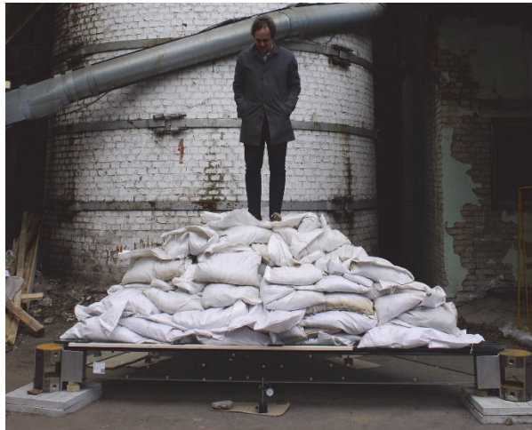
Fig. 12: Full Scale Testing of Glass Beam, Nodes and Panels
