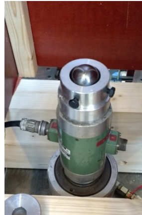
Fig. 13,14,15 Hydraulic piston, force gauge, ball joint.
