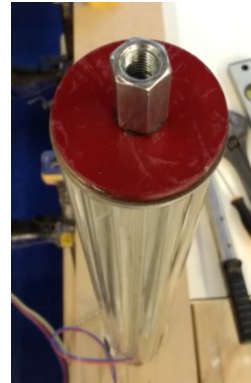
Fig. 10 extension nut to apply pre-stress
