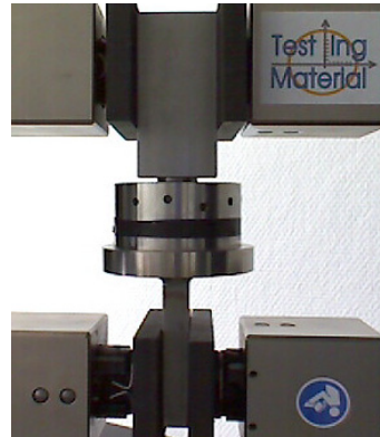
Figure 2: Photograph of point support specimen.
