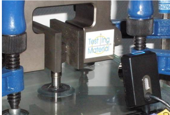
Figure 11: Test set-up for point support P1.
