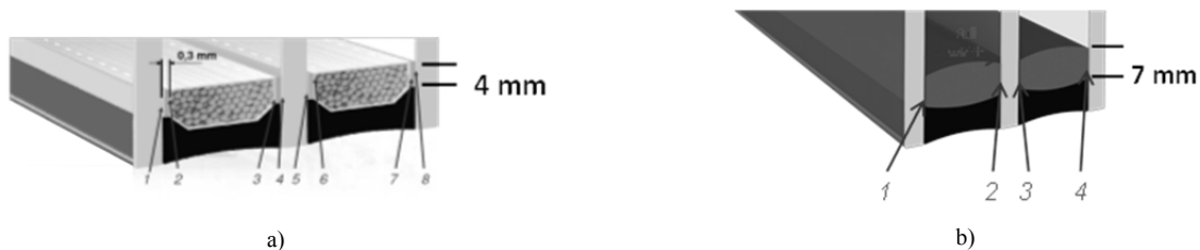
Fig. 27 Number of boundary layers and diffusion/permeation pathways a) conventional b) Ködispace 4SG
