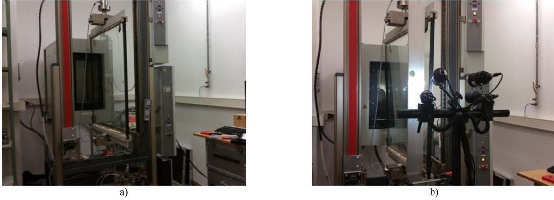
Fig. 20 Test assembly for the torsion tests with 1 000 mm x 1 000 mm IGUs; a) no load applied; b) M = 200 \text{ Nm}
