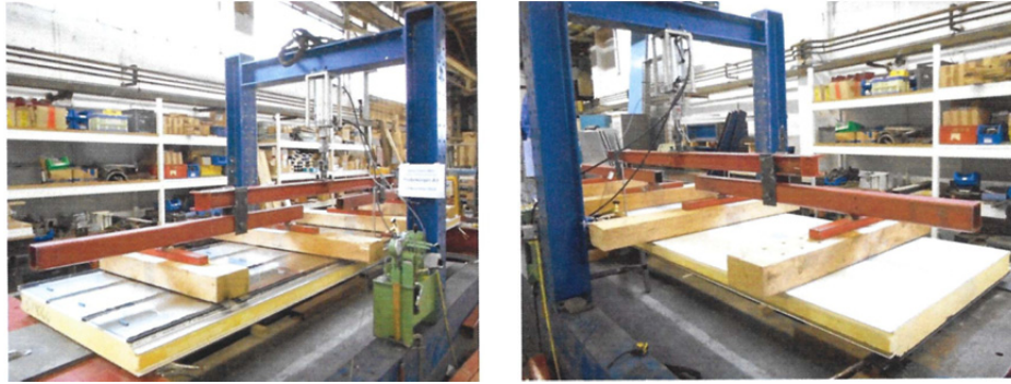
Fig. 8 Bending test of glass sandwich panel in accordance with EN 14509 with bonded transparent glass ply at top (left) and bottom (right) of sandwich panel.
