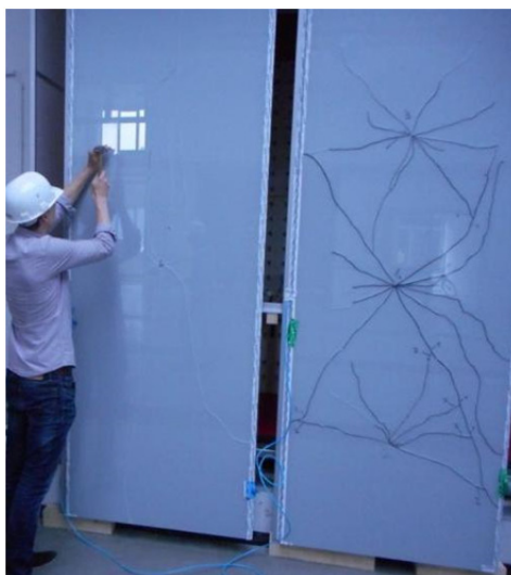
Fig. 11 Breakage pattern of heat-strengthened glass ply bonded to a sandwich panel.
