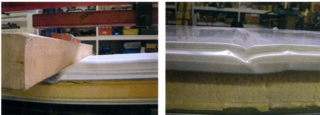
Fig. 9 Compressive failure of face sheet (crumpling); glass ply is bonded to bottom face sheet.
