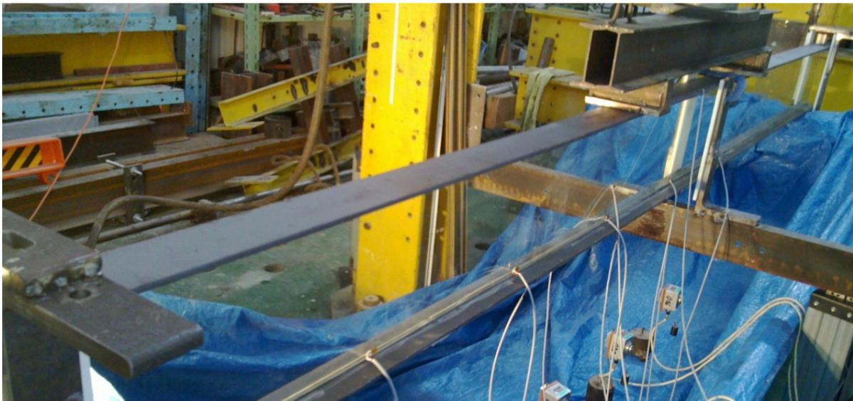
Fig. 10 Hybrid steel-glass beam.
