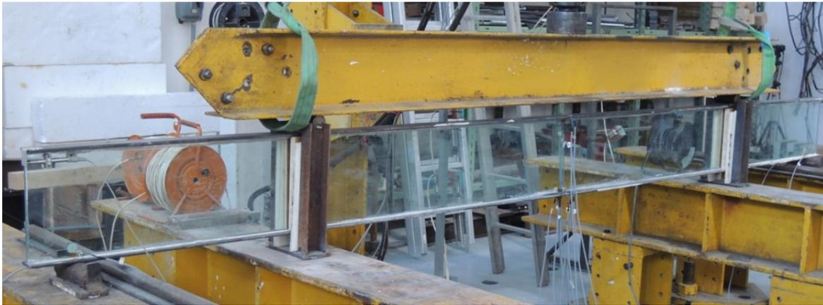
Fig. 12 Hybrid steel-glass beam with SikaFast-5211 NT.
