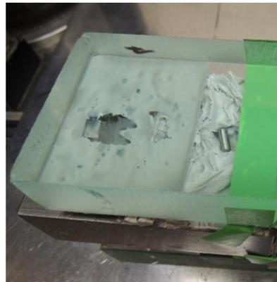
Fig. 6 SikaFast-5211 NT failure mode.
