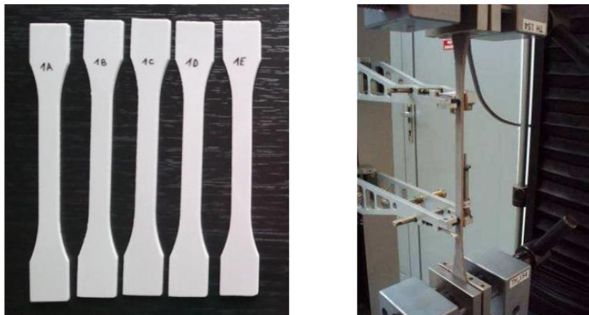
Fig. 1(a) Shape of test specimens, b) Specimen during tensile test.
