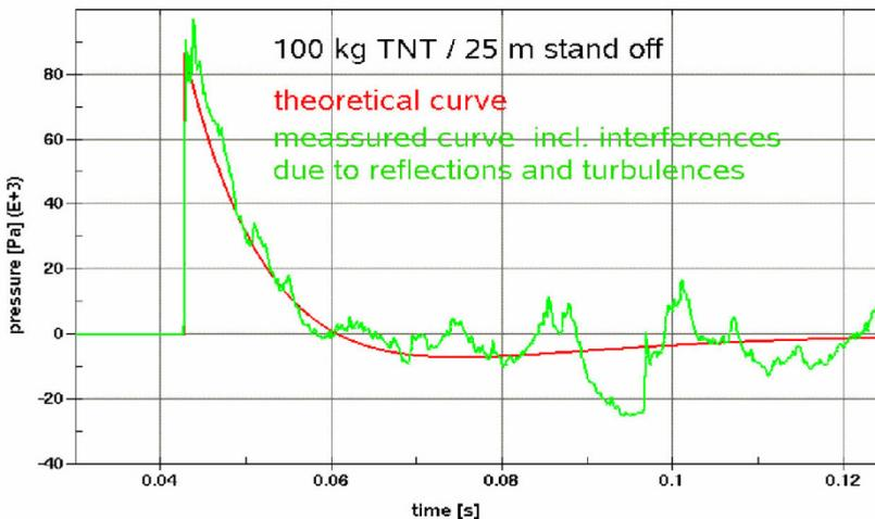
Figure 8. Measured and computed pressure-time-curve (measurement source: Bollrath Pro FORCE) [6].
