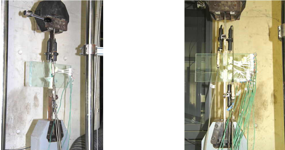
Fig. 12 Simple shear tests setup
