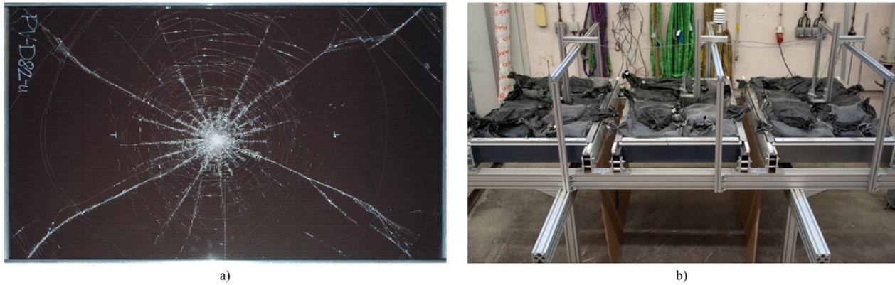
Fig. 11a) Typical fracture pattern of the a-Si/μ-Si superstrate modules (front view) before load application; b) Test rig for the winter scenario at room temperature.
