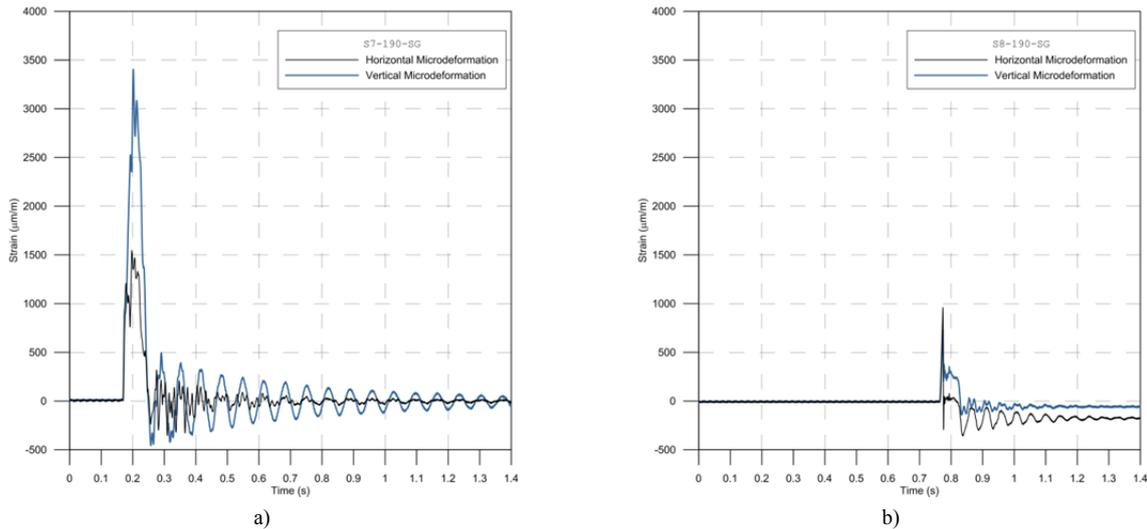
Fig. 3 a), b) Strains vs. time diagrams for S7 and S8 panels, respectively, subjected to impact at a drop height of 190 mm.
