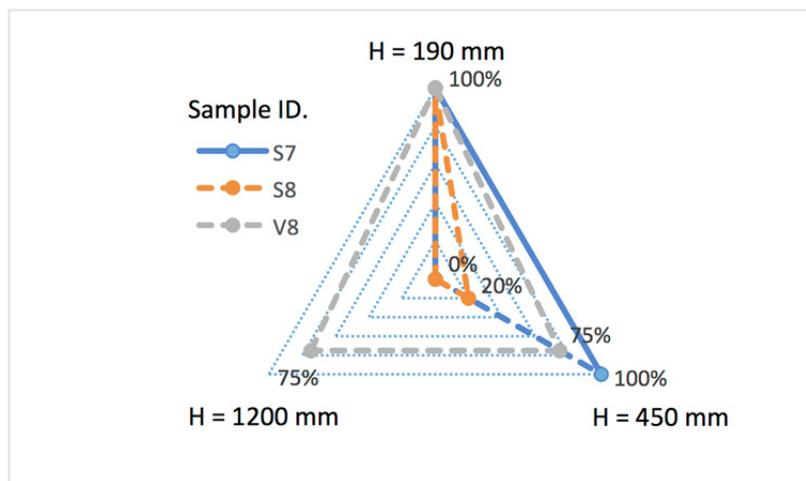
Fig. 4 Percentage of specimens passing unbroken the impact test at different drop height (H).
