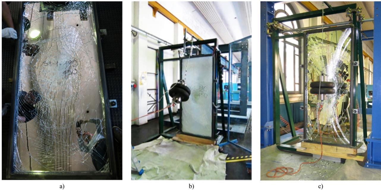
Fig. 2 S8, V8 and R8 panels following impact at a drop height of 450 mm ( a), b) and c), respectively).
