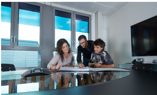
Fig. 12 Offices in Neuchatel equipped with EC glass and in-pane zoning. The upper zone is in the fully tinted state to block glare while the lower zone is in the clear state to admit sufficient daylight. Views to outdoors are maintained all the time. ©Vetrotech Saint-Gobain.
