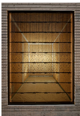
Fig. 3 Prototype of the structured switchable glazing in a façade test facility. TN-cells partially darkened. Phot.: J. Rettig, ILEK
