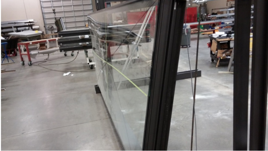
Fig. 5 Photo of Buckled Glass from Previous Testing by Enclos
