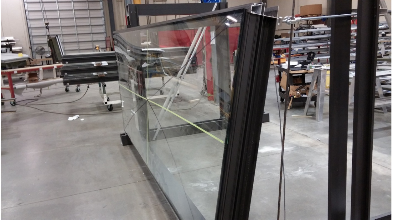
Fig. 7 Cold Formed Test of 1525mm x 3658mm Glazed Frame.
