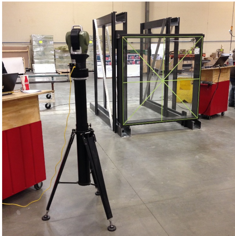
Fig. 8 Laser Tracker Station and Adjustable Cold Formed Testing Apparatus.
