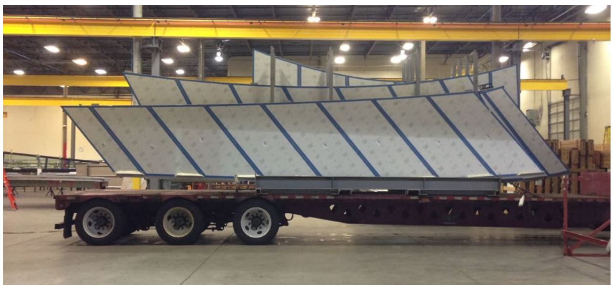
Fig. 3 Sloped Façade Units.
