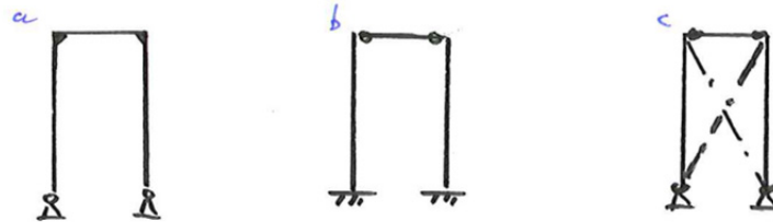
Fig. 8 Options for structure of wings: a = portal, b = clamped columns, c = bracings.
