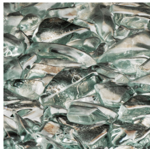
Figure 4: Fused glass shards – irregular arrangement, long heat exposure.
