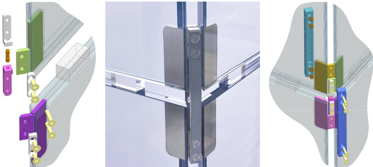
Fig. 9 Edge connection between four façade panels, self-stabilizing.
