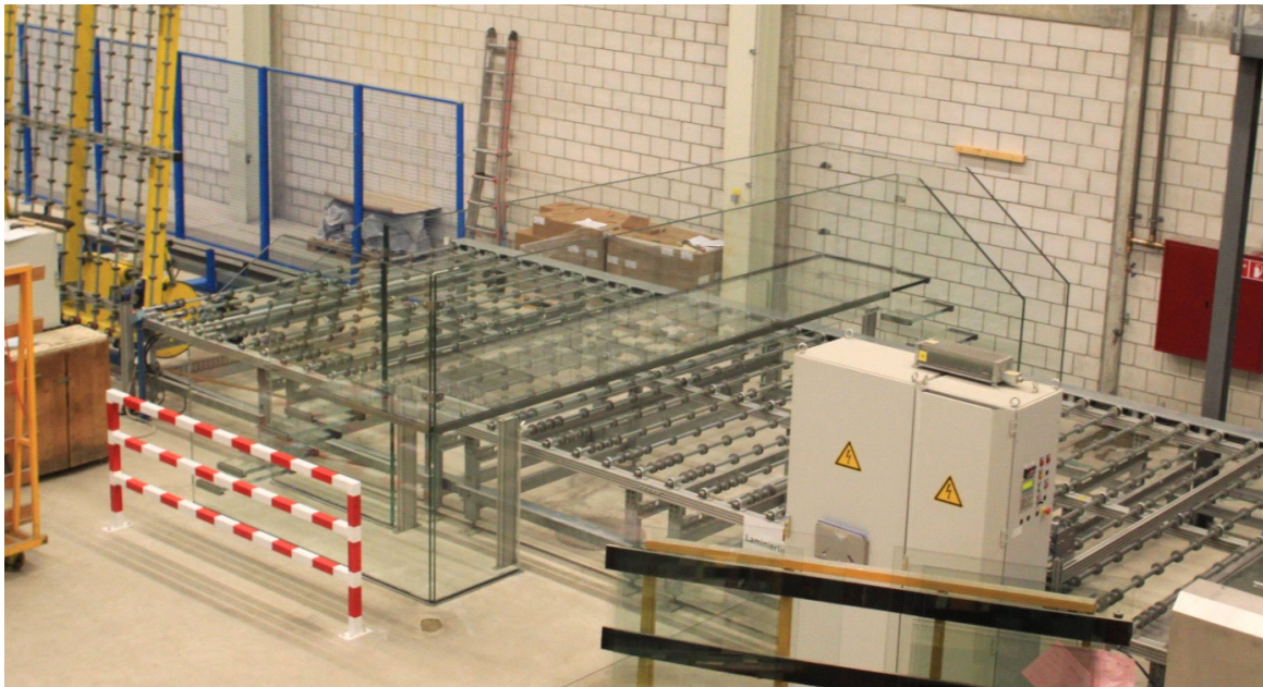
Fig. 5 Pilot Project of a full glass bridge with structurally bonded connection elements.
